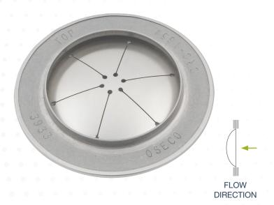
OsecoElfab's CRC is a metal disc with a 3.125" outside diameter. The CRC fits the standard threaded or bolted railroad tank car safety vent. Should vacuum occur during unloading or while the car is in transit, the stainless steel vacuum support protects the seal.
