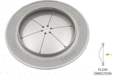
OsecoElfab's CRC is a metal disc with a 3.125" outside diameter. The CRC fits the standard threaded or bolted railroad tank car safety vent. Should vacuum occur during unloading or while the car is in transit, the stainless steel vacuum support protects the seal.
