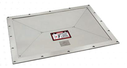
The OsecoElfab GLVF is an excellent solution for protecting bucket elevators during deflagrations. The lightweight vent features a built-in gasket and built-in outlet frame that eliminates the need to fabricate an angle iron hold down frame.
