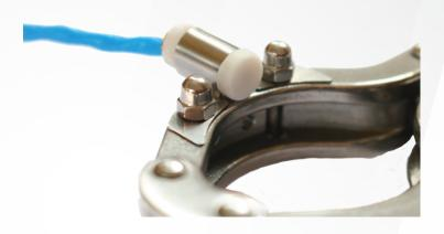
Vent-Tel is designed to fit OsecoElfab's sanitary rupture discs. Unlike membrane-type detectors, Vent-Tel is an independent, reusable solution. It is mounted outside the process and does not come into contact with the process media. This removes risks associated with contamination, false alarms due to pressure fluctuations, and leakage.
