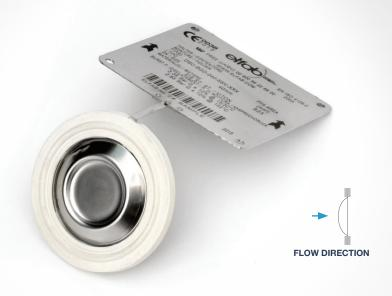
Bio-Gard is a low-pressure, peripherally scored, reverse-acting rupture disc designed specifically for protection of aseptic and hygienic plant.
