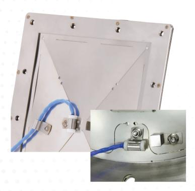
When fitted to explosion panels, Vent-Tel provides an instantaneous signal of panel actuation within any application. Operating via a simple N/O reed switch and magnet technology, the detector can trigger a safe and rapid shutdown of the process should an overpressure event occur.
