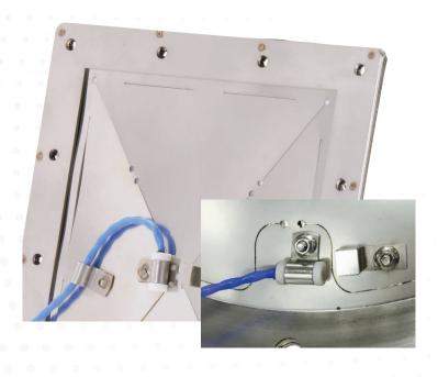
When fitted to explosion panels, Vent-Tel provides an instantaneous signal of panel actuation within any application. Operating via a simple N/O reed switch and magnet technology, the detector can trigger a safe and rapid shutdown of the process should an overpressure event occur.
