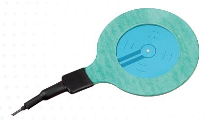
With a thickness of just 3/16", OsecoElfab's SVT rupture disc sensor is designed to be installed on top of existing rupture disc assemblies. The SVT is installed on the vent side of the rupture disc assembly and is the preferred sensor model for use upstream of safety relief valves.
