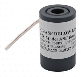
The ASF has been designed for use in the paper and plastic manufacturing industries. Should a rupture disc burst, the sensor sends an immediate alarm signal for rapid recognition of the failure. Steps can then quickly be taken to restart the process and minimize product loss.
