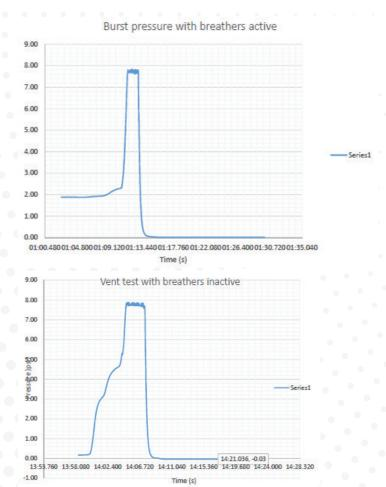
The test disc was rated for a burst pressure of 7-9 psi. This is the standard configuration with the PRO-LP disc, as pictured on the front page.
