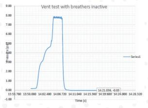
The test disc was rated for a burst pressure of 7-9 psi. This is the standard configuration with the PRO-LP disc, as pictured on the front page.
