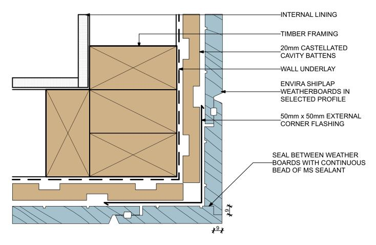
50 mm MIN COVER OF FLASHING BEHIND WEATHERBOARD
