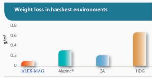
Measurement of mass loss pH: 11.7 - Solution with 5% NH<sub>3</sub> - T: 20°C - Test duration 24 h
