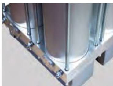
Detail of modular PSA aluminum banks, based on single modules concept.
