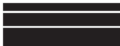
**Recommended thicknesses** for tiles for application with glue: tile area up to 0,72 sqm - 12mm. For greater areas - 20mm.
