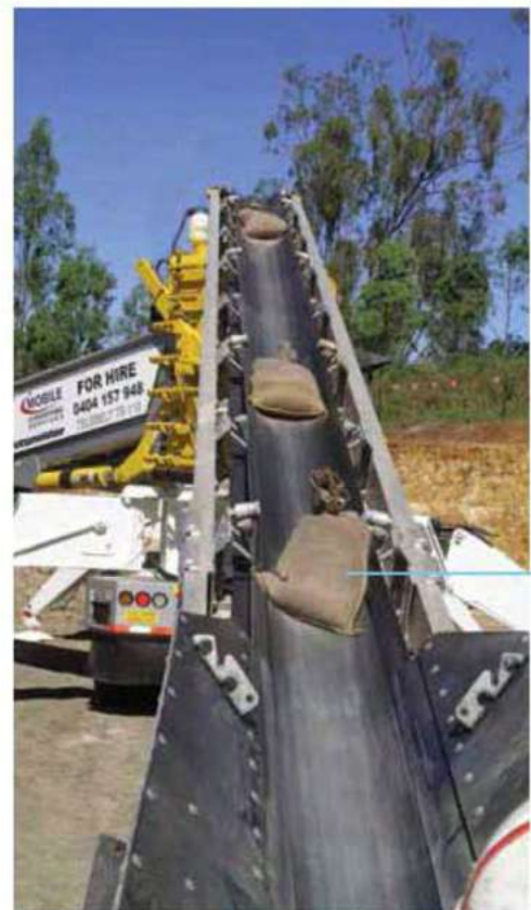
Placing soil on a noise wall: a productive alternative to other methods in areas that cannot be accessed directly or safely. Mulch and bark can also be placed, and belt speed and discharge height can be adjusted to suit cellular confinement systems.
