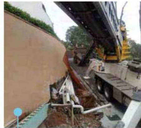
Flexible options for positioning outriggers allow this Telebelt to set up in an area with restricted access.
