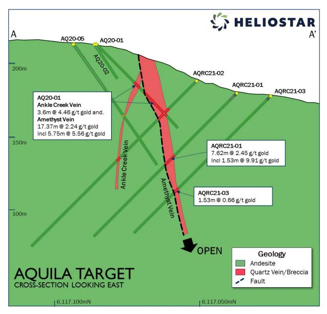
Figure 2: Aquila cross section looking to the east.
