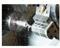
Wet machining or drilling is preferred for ceramic materials, in order to keep the workpiece and tool cool (to extend service life) the material.
