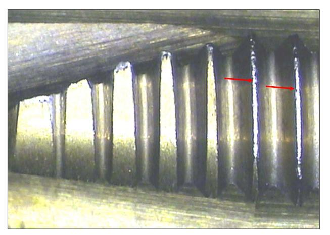
Wear on the first full tooth facilitates wear at the second tooth, etc.
