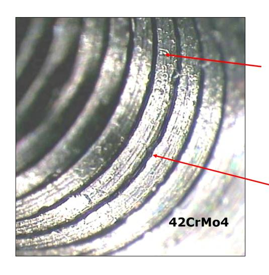
Creation of burrs in the core of the internal screw thread particularly when the screw taps wear more in the core due to hardening of the core holes
