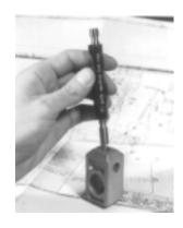
and maximum pitch diameters for internal and external threads. It is important to remember that classes of thread actually represents manufacturing tolerances. The closer the tolerance required, the higher the cost involved in producing the parts. Therefore, designers and engineers should always try to select the class of thread with the widest permissible tolerance.
