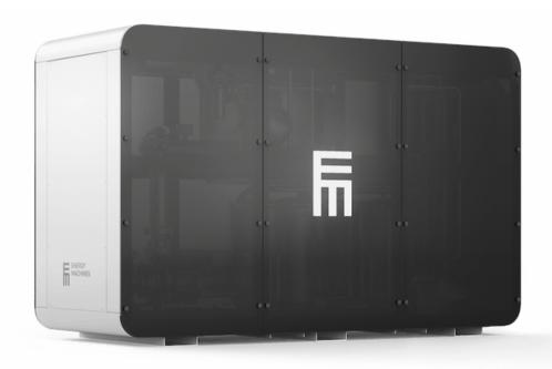
This Energy Machines™ EMHP model contains two refrigerant circuits with a semi-hermetic reciprocating compressor in each. Together with optional frequency inverters, the EMHP model has the capability of providing either high turndown or extra capacity when required. The two refrigerant circuits are completely independent, ensuring the stability of the heating supply.
