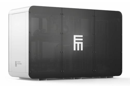
This EMA Energy Machines<sup>™</sup> model contains two circuits with a twin compressor in each. It includes a subcooling system enabling the efficient recovery of heat energy between the condenser and expansion valve. This results in higher performance due to a greater energy uptake in the machine's evaporator process.
