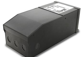
ParadigmLED's PL-PS-M300-DIM-24 is a multioutput class 2 LED dimmable LED driver. It is equipped with push-to-reset breakers, one on each output, protecting both the load and the driver. Encased in a high-quality NEMA 3R metal case enclosure, that includes 5 knock-outs to enable easy installation. THe PL-PS-M300-DIM-24 is dimmable with any standard MLV TRIAC dimmer.
