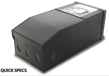
ParadigmLED's PL-PS-M200-DIM-24 is a multioutput class 2 LED dimmable LED driver. It is equipped with push-to-reset breakers, one on each output, protecting both the load and the driver. Encased in a high-quality NEMA 3R metal case enclosure, that includes 5 knock-outs to enable easy installation. The PL-PS-M200-DIM-24 is dimmable with any standard MLV TRIAC dimmer.
