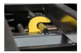
Each set of hooks must be undamaged, working correctly, and the container must be locked onto the chassis.
