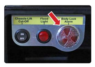
4. The in-cab alarm must work properly. When container is unlocked the alarm sounds and flashes.
