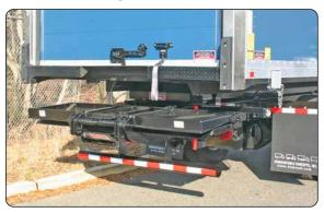
If applicable, unlock and lower the lift gate so it clears the container when backing under it.
