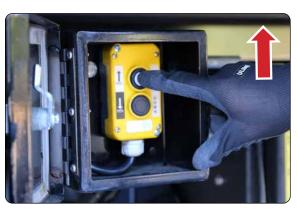
12. Walk to the control box and press the up button to raise the lift until all four legs are off the ground.
