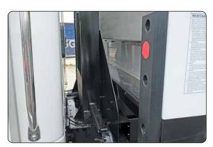
10. Go to the front of the container and check to be sure the steel plates are touching the chassis lift's wing plates. If they are not touching it will be very difficult to properly lock the container on. If necessary, reposition the truck.
