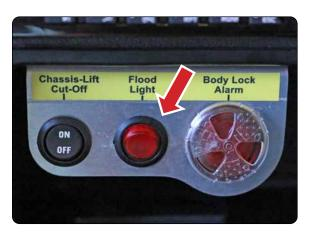
4. Your truck is equipped with two flood lights operated by a switch located near the incab warning buzzer. Turn them on before backing up.
