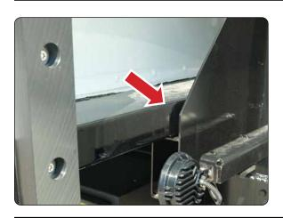
**8.** The best time to check alignment is after rear tires pass the front legs.
