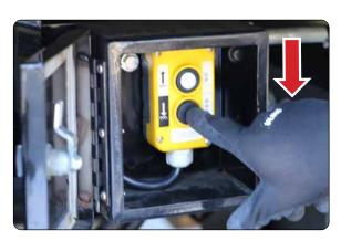
Return to the control box and lower the lift assembly by pressing the down button in the control box.
