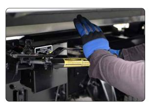
19. When the locking bar is fully raised the spring-loaded safety handle will move into place.
