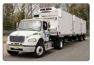
3. Line-haul tractor-trailer that mounts, demounts, and line-hauls multiple containers to a remote location.
