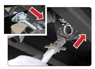
22. Remove the light plug from the holder and plug it into the receptacle
