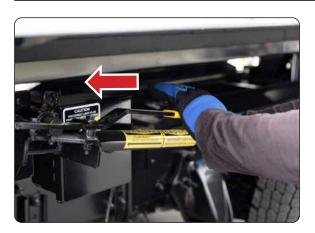
7. Push the safety handle inward to release the locking assembly.
