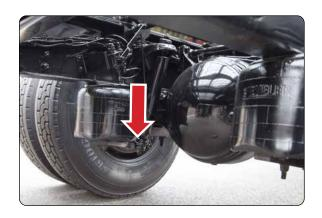
3. In some cases, lowering the air suspension before demounting will result in lower standing heights to get the container's floor closer to dock height
