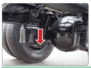
**6.** If you dumped your air suspension during the demounting process, be sure the air suspension is lowered.
