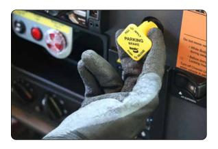
Inside the cab, start truck, and engage the parking brake
