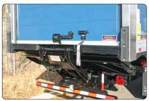
24. If your truck is equipped with a lift-gate raise and lock the gate in its normal ride position.
