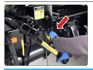
8. Lower the locking bar by pushing it down.
