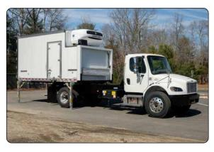
21. Return to the cab of the truck and pull straight out until the chassis is clear of the container.
