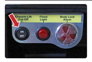
2. Press the chassislift power button on the dash
