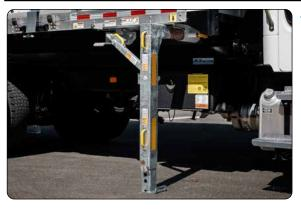
16. The support leg is only securely locked when the leg brace and the spring bolt pin are engaged.
