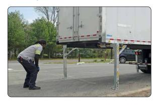
5. Line up the truck chassis so it's straight in line with the guide rails at the front of the container.
