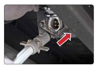
**3.** The light plug must be plugged into the container and lights must be functional.
