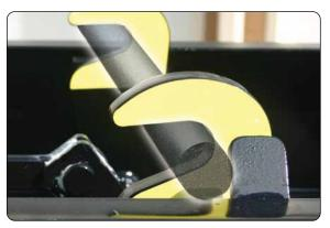
23. Confirm that the container is locked onto the truck by visually checking that locking hooks are securely attached to the locking bars on the underside of the container.
