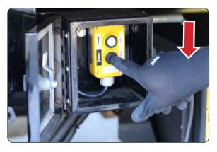
17. Return to the control box and lower the chassis lift until it is completely down on the truck frame.
