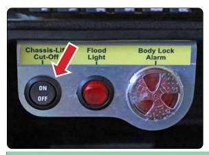
**9.** Set the parking brake, put the truck in neutral or park, and keep the engine running. Be sure the power button is in the on position.
