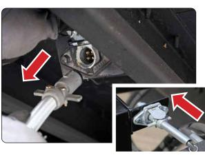
19. Double-check to be sure the light plug is disconnected from the container and inserted the storage holder.
