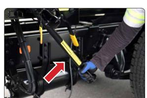
18. Lock the container onto the truck by raising the locking bar to engage the locking hooks.
