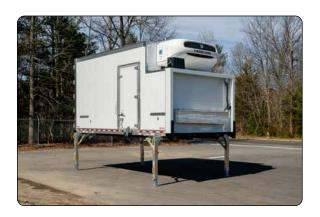
Demountable containers standard truck bodies equipped with retractable legs.
