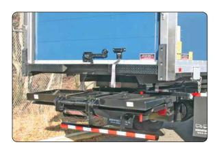
4. If applicable go to the rear of the truck and unlock and lower the lift gate so it clears the container when pulling the truck out from under a standing container.
