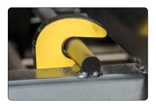
1. Visually confirm container is properly locked onto the truck chassis. The hooks on the locking mechanism must be engaged over the locking bar on the container.
