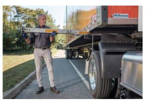
14. Lift the vertical portion of the leg to a horizontal position and slide the entire leg into the leg housing.
