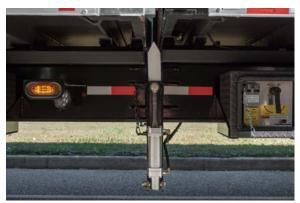
Driver- and passengerside center-stops must be raised.
