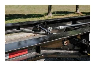
2. The locking hooks must be in the unlocked and down position.
