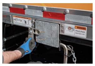
All legs must be properly stowed with leg pins secured.
