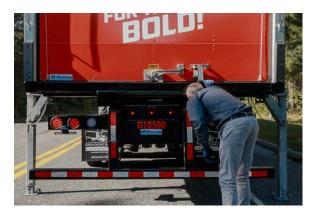
19. Walk to the rear of the trailer and check that there is proper clearance between the container's long rails and trailer's main rails.
