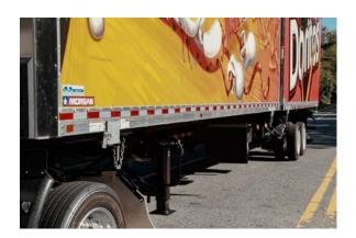
17. Work your way around the trailer to the driver side until all eight legs are stored and secured.
