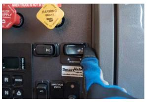
18. Return to the tractor's cab and lower the air suspension by pushing the air suspension toggle switch to lower.
