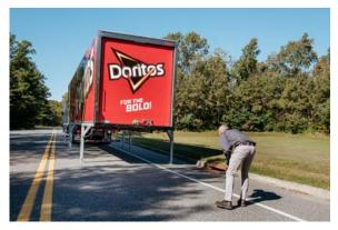
3. When the rear wheels of the trailer are under the front container get out of the tractor and check alignment.
