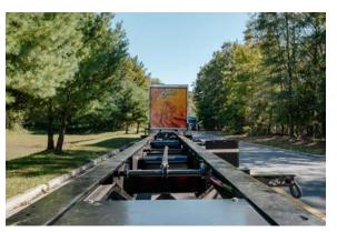
Before backing up make sure the trailer is linedup to go straight under the containers.
