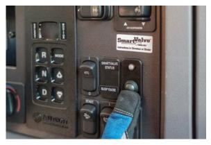
9. Raise the tractor suspension fully by pushing the "suspension raise" button on the dash for one second.
