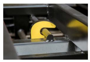
Visually confirm both containers are properly locked onto the trailer.
