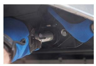
Be sure both light plugs are inserted into their receptacles and both containers have working marker lights.
