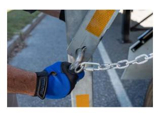
**14.** Insert the leg pin through the brace and leg. Swivel the handle down to secure it.
