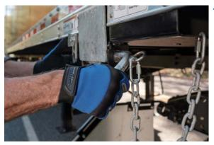
**12.** Rotate the handle portion of the leg pin upward and slide it out of the leg and retainer.
