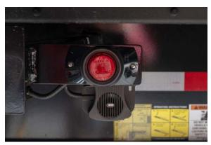
**12.** The exterior alarms and lights will turn off when both containers are properly locked onto the trailer.
