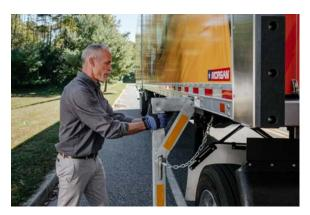
**15.** Push the leg assembly into the housing until the top brace touches the container side rail
