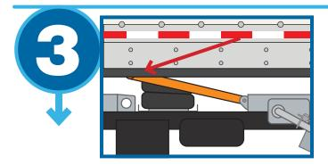
Raise front and be sure air lift device is in the guide rails.
