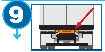
LOWER rear air lifting device and be sure container is nested OVER the chassis.
