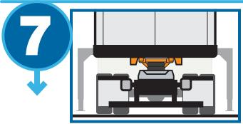
Raise REAR and be sure air lift device is in the guide rails.
