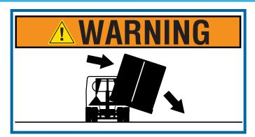
An improperly secured container that falls off a chassis can result in injury or death. It is the driver's responsibility to make sure that the container is properly locked onto the chassis before each trip.
