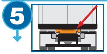
LOWER front air lifting device and be sure container is nested OVER the chassis.
