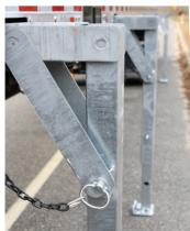
3. Confirm all 8 container legs are deployed and secured with pins
