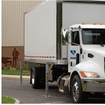
2. Confirm all 4 container legs are deployed and secured with pins
