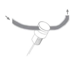
The IRt/c.01HB model pictured, actually measures the internal fluid temperature by measuring both tubing surface and ambient temperatures then calculating the internal temperature necessary to maintain the heat balance. A convenient clip head provides a reproducible mounting location for the sensor and can be quickly attached to new tubing and removed from used tubing.
