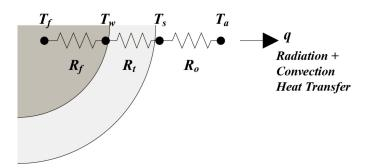
$$q = \frac{1}{R_f + R_t + R_o} \left( T_f - T_a \right)$$
