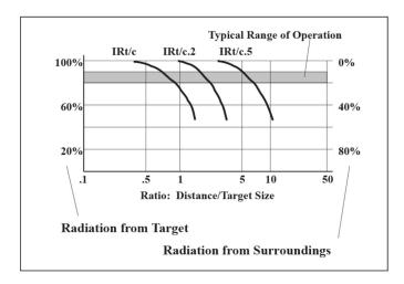
Under typical conditions, placing the IRt/c such that the target exactly fills the field of view results in approximately 80 to 90% target signal, and 10 to 20% surroundings signal.
