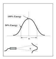
A common convention in infrared thermometry, and the one used to verify the optical performance of IRt/c's, is to define the field-of-view by the "1/2 energy points" in an optical traverse experiment. The resultant data looks like a "Bell Curve" as indicated in the illustration. The field-of-view is simply the angle between the 50% energy points.
