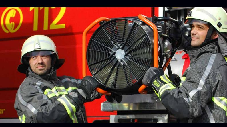
High performance fans allow effective ventilation of burning buildings and sites of operation from smoke, heat and toxic gases. The conditions for the fire fighters are significantly improved. The attack group can orient itself faster inside the object and fight the fire more effectively.
