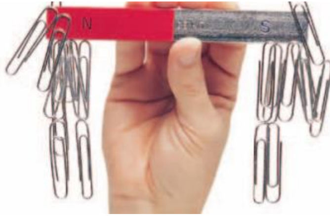
Figure 1 More paper clips stick to the ends, or magnetic poles, of a magnet because the magnetic effects are strongest there.
