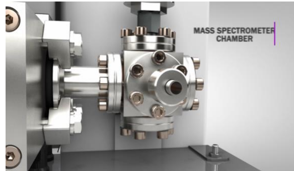
Figure 3 – Mass Spec sensor enclosed in a 1.33" CF manifold attached to a turbo pump
