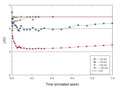
The reduction values (LRV – log reduction value) remain relatively stable over the time frame. It should be noted that even though the filter is rated at 0.05 micron, capture efficiency of 0.03 micron particle is quite high.
