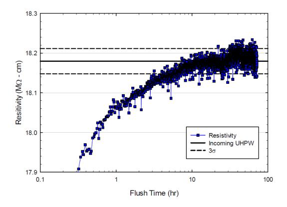
In production, each ZTEC-E filter is flushed with semiconductor grade UPW for 50 minutes at a flow rate of 10 GPM, assuring the high purity of each filter shipped. For on-site purposes, customers are advised that a rinse-up of no more than 35 minutes at a flow of 3GPM will achieve 18 megohmem resistivity.
