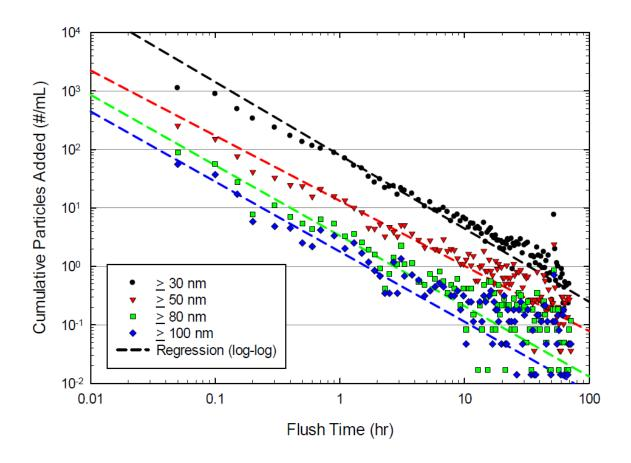
In production, each ZTEC-E filter is flushed with semiconductor grade UPW for 50 minutes at a flow rate of 10 GPM, assuring the high purity of each filter shipped. For on-site purposes, customers are advised that a rinse-up of no more than 120 minutes at a flow of 3 GPM will achieve single digit particle counts.
