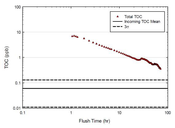
During manufacture, each ZTEC-E filter is flushed with semiconductor grade ultrapure water for 50 minutes at a flow rate of 10 GPM, assuring the high purity of each filter shipped. For on-site purposes, customers are advised that a rinse-up of no more than 60 minutes at a flow of 3 GPM will achieve single digit TOC level.
