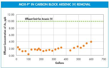
Arsenic reduction with a narrow diameter carbon block. Targeted performance, 300 gallons.
