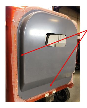
Since this day cab conversion kit installs on the inside flange, there is no need for removing outer ring of hucks.
