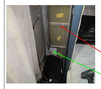
Before removing sleeper you should unbutton interior trim boot from cab and save to use with interior pieces later on. This trim boot will make the 5 ½" transition on the sides of the "XL" kit.
