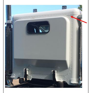
The Unibilt Economy can slide under cab roof, lay on top of cab roof and putty gap, or you can trim the cab roof to fit flush.
