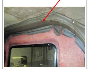
You need to re-snap the interior boot trim that went between the cab and sleeper in place. You should cut off some excess as you see fit. Trim away back side buttons and flatten out to make a smooth surface to sandwich between fiberglass and Daycab Company interior panel. Attach the loose tabs of the boot to the kit using spray glue or whatever you think is appropriate.
