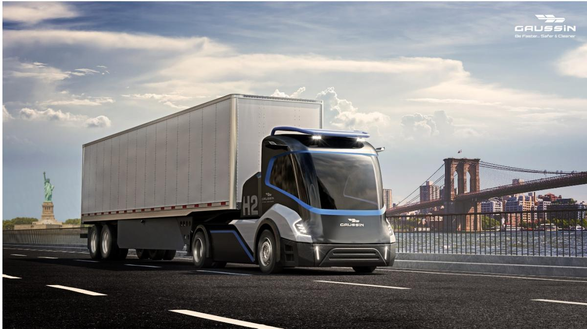
Autonomous road tractor with electric and hydrogen propulsion, capable of towing 44 T semi-trailers
