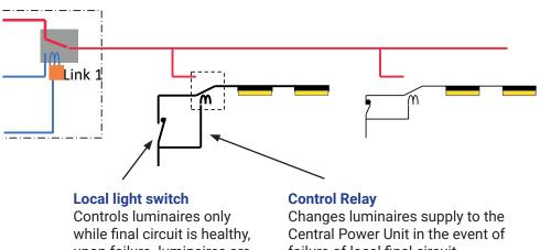
upon failure luminaires are automatically connected to maintained emergency output failure of local final circuit
