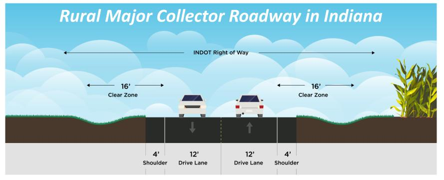
55 MPH Design Speed (45 mph posted speed) with 5% Maximum Vertical Slope and minimum horizontal curvature
