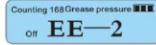
8 Alarm due to insufficient filling (It has no influence on system operation. Fault will be automatically cleared at the time of next normal operation)
