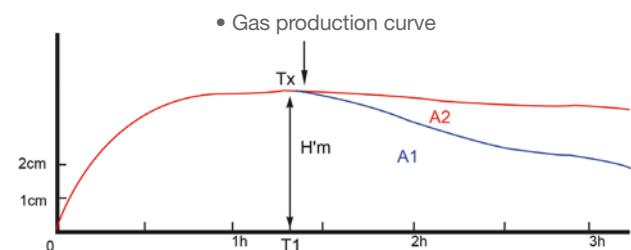
The gas production curve enables the user to determine the retention coefficient R (the comparison in % between the volume retained within the dough and the total volume of gas produced during the test).
