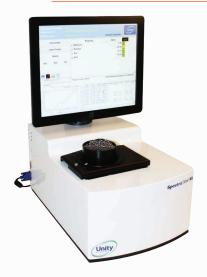
NIR analysis is a proven technique that provides simultaneous results for moisture, protein, fat, fiber, ash, and other parameters in under a minute. The speed of analysis allows 100% measurement of incoming oilseeds, in-process meals and final products. Raw ingredients suppliers can be verified to ensure they are providing quality materials, and to flag out of specification loads for claims. The use of NIR ensures consistent quality in meals and can maximize return from the feedstock.
