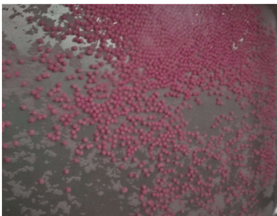
Lyobeads in liquid nitrogen after dispensing
