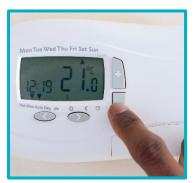
**Set the thermostat to between 18 - 21 °C.** This means that your boiler will heat up the air to this temperature and no more. The ideal temperature varies per room use but should sit somewhere within this range to be comfortable. Every degree warmer than this can increase your energy use - and bills - by 10%!
