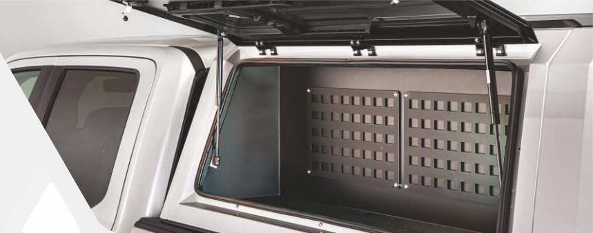
Full-Bin : Fills the entire side opening and provides Molle plates to secure cargo.
