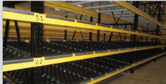
CARTON FLOW First-in-first-out (FIFO) storage for smaller product
