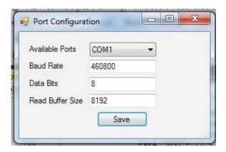
Please Note: You must ONLY change the COM port number. DO NOT adjust any of the other settings! Click on the drop-down box labeled "Available Ports" and select the COM port used by the instrument. If there is any doubt about which COM port is correct, consult the Windows Device Manager for details. Select the appropriate COM port, and press 'Save'.
