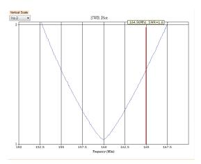
Note also the horizontal frequency scale along the bottom, in MHz, and the vertical scale control, top left. While the frequency scale is fixed (it's determined by the frequency range you chose when you calibrated the instrument), you can use the vertical scale control to change the appearance of the chart to get the best view of the trace.
