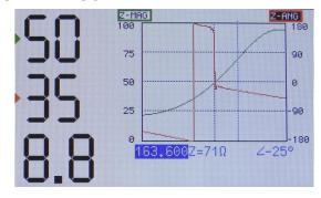
The VNA screen (shown here in narrow format) will allow you to directly view impedance magnitude and phase characteristics of virtually any single-ended device. Keep in mind that the instrument must be calibrated (either broadband or frequency-specific) as when doing RL and SWR measurements. The calibration process is identical, and occurs whenever center frequency or span is changed (when in frequency specific mode).
