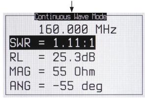
When the MRI-3000 is in Continuous Wave mode, only the Center Frequency will be transmitted. Eliminating the Swept Frequency eliminates the need to graph the results and only values at Center Frequency are posted as a digital result. This permits faster viewing of any changes during DUT tuning being performed. To exit press the Sweep/CW key again to return to the previous testing mode and the swept measurements will resume.
