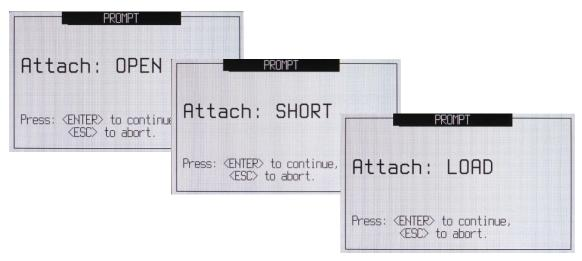
Pressing ENTER after the Load is attached completes the calibration process for single-port measurements, and will return the MRI-3000 to the previously selected measurement screen.
