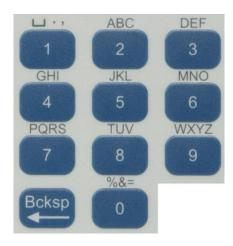
The alpha-numeric keypad operates like those on smaller cell phones. Press a selected key once for entering the number and repeat the key's presses to cycle to the character desired above that key. In an alpha entry screen the first press will present the first alpha character above the number. Subsequent presses will cycle the alpha characters and finally the number or use the Up or Down arrow to cycle through the entire characters set
