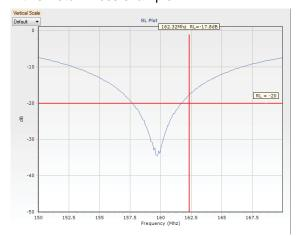
The cursor is at a point on the curve that is above the -20dB limit, and the limit line (at
