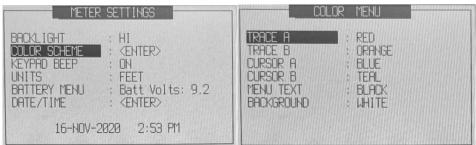
This allows you to adjust the color of the various items on the MRI-3000's screen. When any item on this menu is selected, you can use the (left and right arrow) buttons to select the color for that item from a palette of 16 colors.
