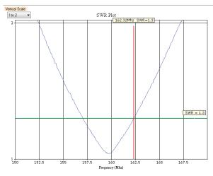
Note that the cursor is at a point on the trace where the value (in this case, the SWR) is at or below the limit line. Note also that the limit line is GREEN.
