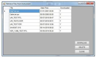
This is a listing of the files in your instrument's file system. The .sys files belong to the system, and should not be downloaded or deleted, unless instructed to do so by support personnel. The .RTL, .SWR, and .VNA, files are Return Loss, SWR, and VNA trace (data) files, respectively. There may also be .SET files, used for storing instrument setups, but those aren't relevant to this discussion.
