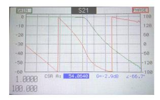
The S21 VNA Screen shown above illustrates how the MRI-3000's Two-port capabilities can be used to analyze a two-port device; in this case, a low-pass filter. Unlike for a single-port measurement, the parameters measured cannot be changed: This always displays GAIN and PHASE (although, the phase trace can be turned off). The cursors work the same as for a single-port measurement, although this display is always in 'wide' format.
